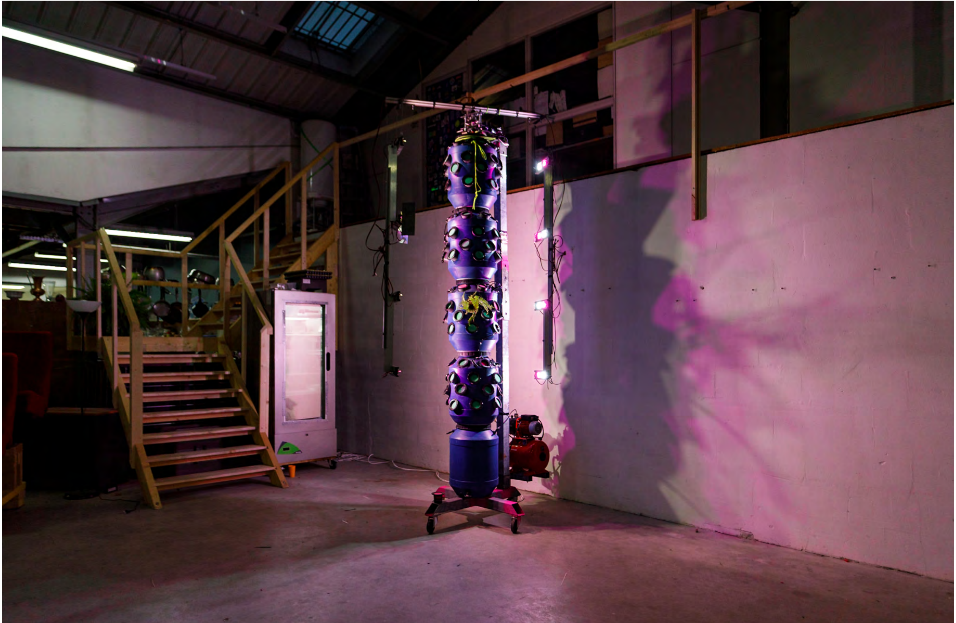
Bootlegg / Hydroponics (LED full spectrum lights, 15 gallon plastic barells, water sprinklers, nutrient solution)
